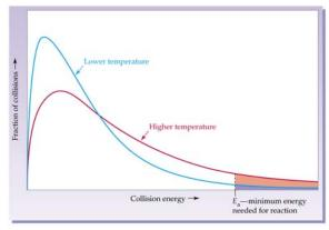
Generally, when the temperature is doubled, the fraction of molecules having high enough E to overcome  $E_a$ , WAY MORE than doubles, which explains WHY the relationship between reaction rate and temperature is NOT linear. It is exponential! Need proof?
