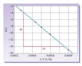
To summarize, if you plot  $\ln k$  vs. the reciprocal of Kelvin temperature, you get a straight line with a slope equal to  $\frac{-E_a}{R}$ .
